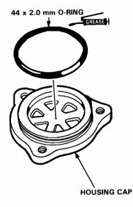
53. Tighten the three 6 mm bolts to secure the housing cap to the gear housing.
